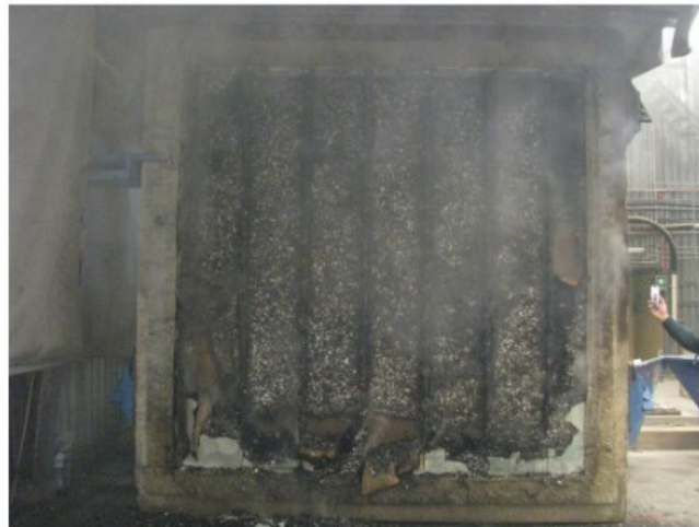
The test specimen after the test. Fire-exposed side.
